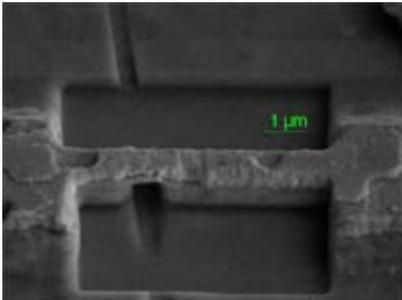
This diagram shows an example of using a beam of gallium ions to cut away a groove in a high-temperature superconductor. This is a scale of about five hundred nanometres and you can see that the ion beams are milling this material with terrific precision; these can be used to do machining of materials on a scale down to about fifty nanometres. A breakthrough in the field came in 1990 when Don Eigler, working at IBM laboratories in Almadon in California, moved individual xenon atoms around on
